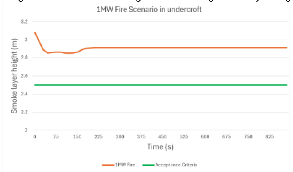
Image – results of the modelling when assessing smoke layer height
